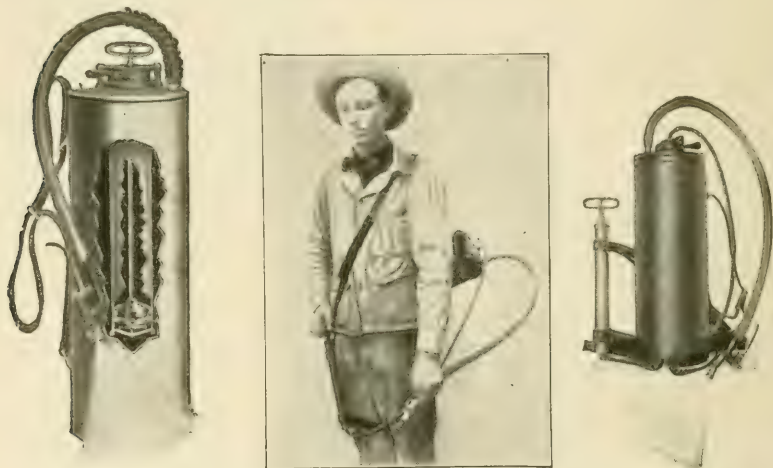
FIG. 32.—Compressed-air sprayer with section of tank removed to show air pump within.
